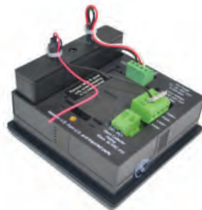
3-8058-3 shown installed in 9900 transmitter
