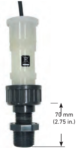
3-2450-A ½ in. union to ¾ in. NPT adapter - PVC material
